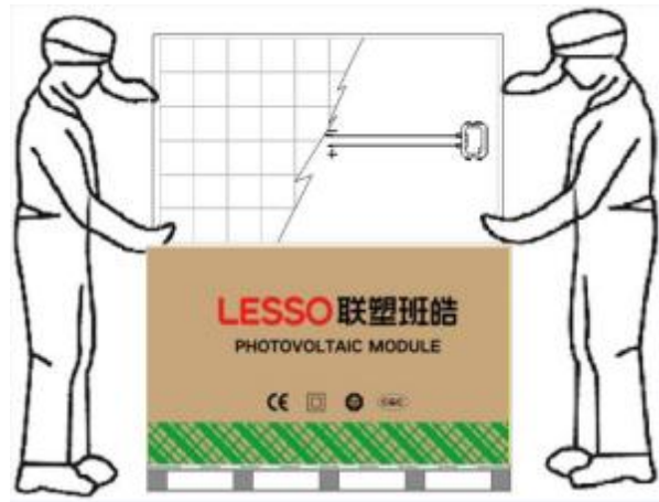
Figure 2 Removing PV modules from a pallet
